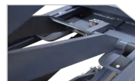
一体式二次举升支撑板 Integrated sub-lift supporting plate
