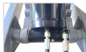
油管爆裂保护装置 Oil pipe broken protective device
